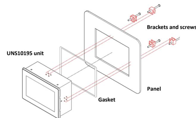
The unit has to be installed in a console with "cutout" of 183 x 135mm , this measure has to be as accurate as possible due to the unit small border profile 200 x 143mm.
