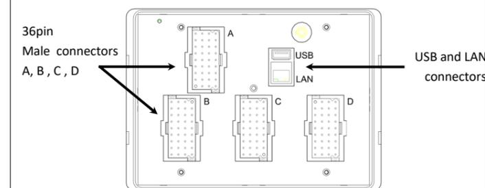
**A-D connectors are not interchangeable.** Each connector (male and female counterpart in optional harness) is marked with a letter from A to D and is polarized using a special stub pin to prevent an wrong connection.
